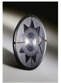
Manger's driver can alone reproduce frequencies from 80 Hz to 40000 Hz, i.e., apart from the two lowest octaves the entire hearing range plus an octave on top of that. The active diameter of the diaphragm is 19 cm, but the higher the frequencies go, the smaller the effective surface area relative to the wavelength to be reproduced.
